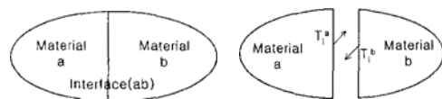
Fig. 1 Interface traction acting on a bi-metallic interface between two region a and b.
